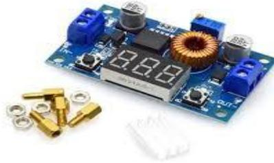
Gambar 2.11 Modul Step Down 12 Volt To 9 Volt
