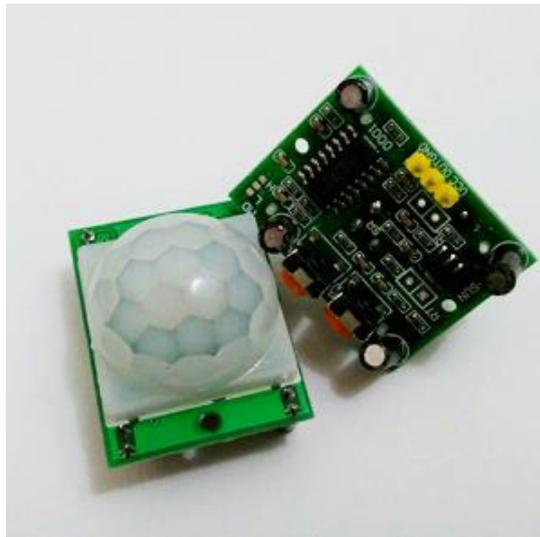
**Gambar 2.5** *Passive Infrared Receiver (PIR)*
