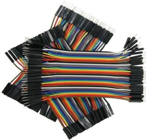
**Gambar 2.9 Kabel Jumper**
