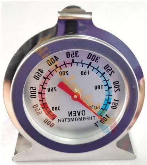
Gambar 2.7 Thermometer Mekanik
