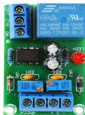
**Gambar 2.10** Charge Modul cut Off
