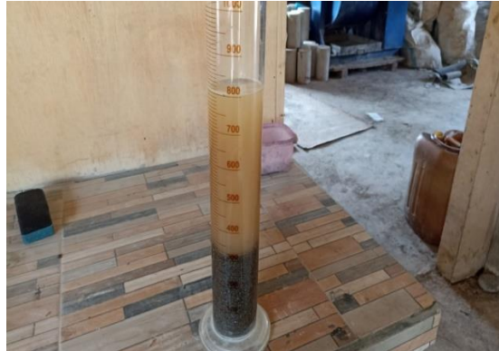
Gambar 3.4 Pengukuran kadar lumpur agregat halus
