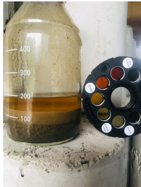
Pengujian kadar organik agregat halus
