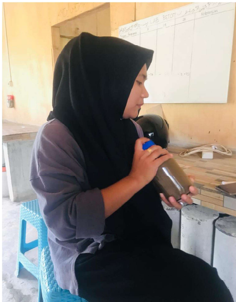
Pengujian kadar organik agregat halus
