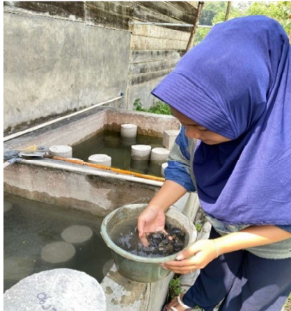
Gambar 4.4 Pengukuran kadar lumpur agregat kasar
