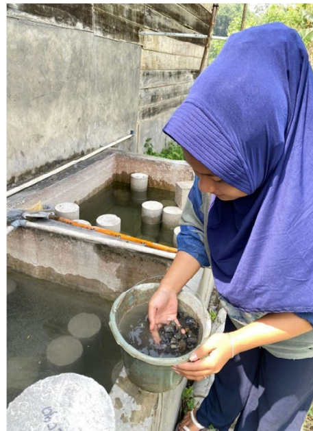
Pengujian kadar lumpur agregat kasar
