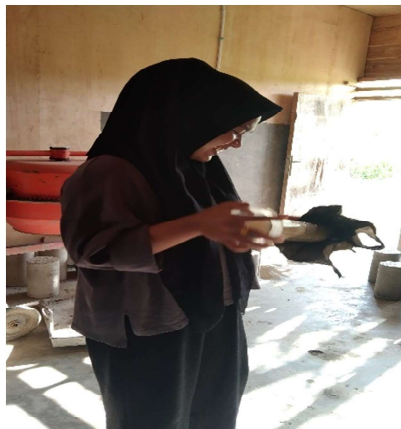
Gambar 4.3 Pengukuran kadar lumpur agregat halus
